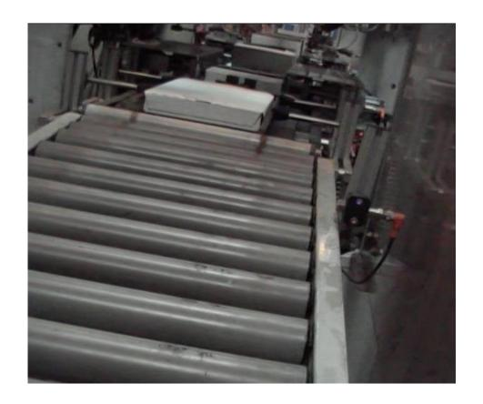
Separate line to handle B2C orders – the parcel is automatically levelized up to the content.
